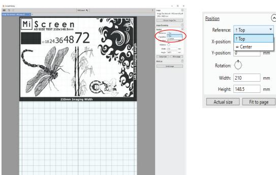
When using the MiScreen A5 Design Frame, any image below 150mm in the lower half of the work area will not be created, as the TPH Stop Hole in the Frame Mount will stop the screen making process. For this reason it is highly recommended to only work in A5 artwork size when using the A5 Design Frame.
