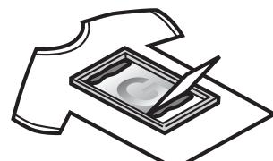
Attaching an imaged screen to the frame and printing with ink on printed materials.
